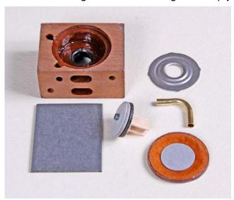
The shoulder where the Pouch Assembly will be glued has been coated with thin hide glue as a sizing, and the inner surfaces and channels of the block have been coated with shellac to reactivate the old shellac seal. The hide glue sizing provides a good bond for the gluing in the Pouch Assembly as well as keeping shellac from interfering with the glue bond.
