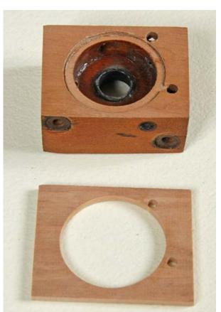
Several pieces of 1/8" thick mahogany were drilled using a 1-3/8" diameter Forestner bit, the same as the Pouch Well, just in case Ron comes across more valves that have to be laminated.
