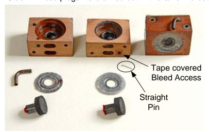
The picture to the left shows two of the three valves after they were taking apart. The front and back have been sanded lightly to level the surface by sanding on a piece of sand paper that has been glued to a flat surface. The valves obviously had been rebuilt before using closed cell foam rubber for the upper and lower valve surfaces. The material has become very hard making most of the valves inoperable. The Fluted Stems do not look original and were too small in
