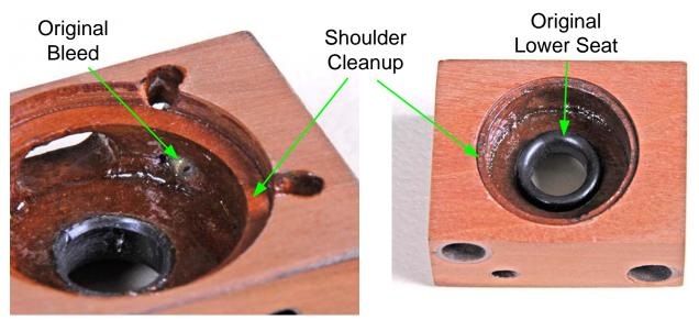
Forestner drill bits were used to clean up the shoulders of both the upper seat and the pouch well. The previous pouches had been glued in with white glue and care had to be taken to remove all the glue without drilling too deeply into the block.
